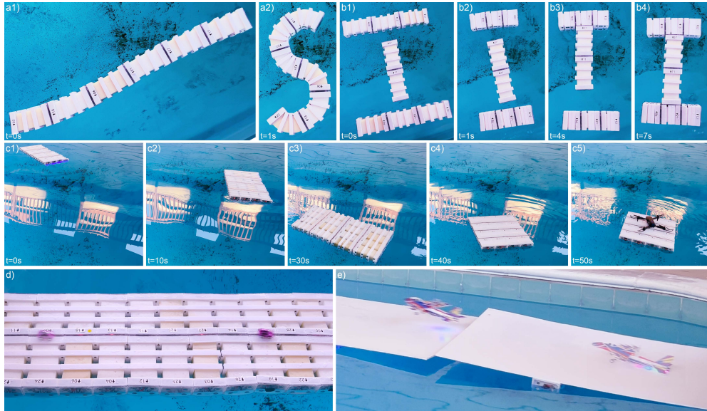
Fig. 4 Structure formation and shape formation of multiple modules. (a) A chain of modules forms an ‘S’ shape. (b) Three chains of modules form an ‘I’ structure. (c) Multiple modules form a soft raft and then compress into a rigid raft, which allows a drone to land on it. (d) A lot of modules form a bridge, allowing a toy car to run on it. (e) Multiple modules form two platforms with a flat board on it. Perform as an aircraft carrier.
